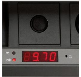
The precise digital measurement readout for the back gauge can be displayed in cm or inches.
