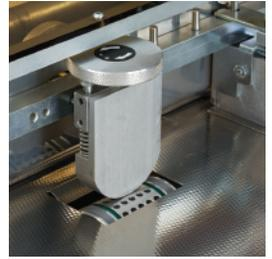
Bottom feed suction allows continuous operation.
