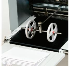
A powered exit conveyor ensures smooth ejection of folded paper.
